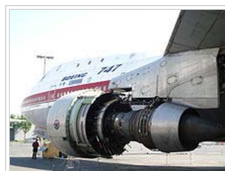
A JT9D turbofan jet engine undergoing maintenance on a Boeing 747 aircraft
