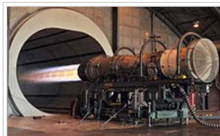
A Pratt & Whitney F100 turbofan engine for the F-15 Eagle being tested in the hush house at Florida Air National Guard base. The tunnel behind the engine muffles noise and allows exhaust to escape
