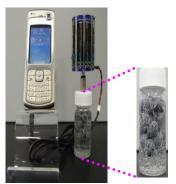
A cellular phone recharged from a 2W PEMFC powered by  $H_2$  produced from catalyzed hydrolysis of NaBH<sub>4</sub> over light-weighted Co catalyst
