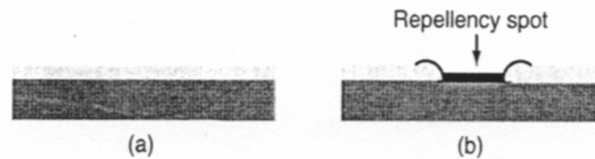
FIGURE 9.5. Even a monolayer of physically adsorbed material can have a disastrous effect on some technological processes, especially critical coating processes in which absolutely smooth, uniform coating is required such as the microelectronics industry. (a) An uncontaminated surface should produce a smooth, uniform coated layer. (b) Surface contamination by a lower-energy material (such as oil molecules) may result in the formation of “repellency” spots or other defects, producing less than optimum or even useless finished products.
