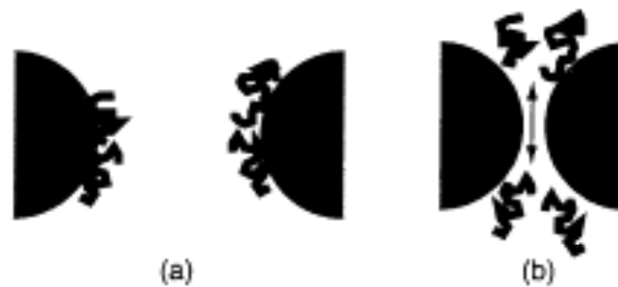
FIGURE 10.12. In a sterically stabilized system containing low-molecular-weight or weakly adsorbed polymer (a), as two particles approach, the loosely bound polymer may desorb, leaving “bare” spots on the approaching surfaces, leading to an enhanced flocculation tendency (b). That process is referred to as “depletion flocculation.”
