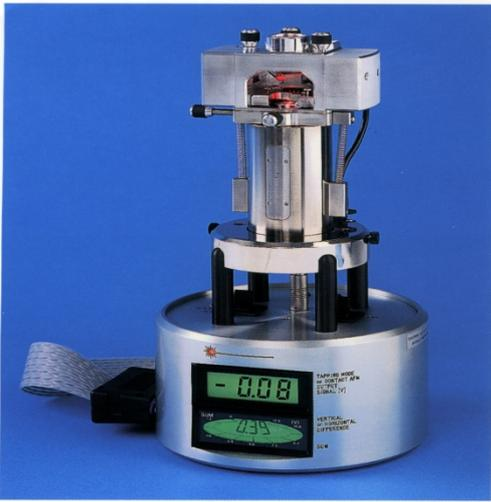
Figure 3: Digital Instruments MultiMode™ AFM, optimized for high resolution force measurements and topographic imaging.
