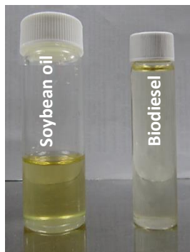
Biodiesel made from catalyzed transesterification of soybean oil in methanol over zeolite catalysts
