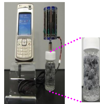
A cellular phone recharged from a 2W PEMFC powered by H 2 produced from catalyzed hydrolysis of NaBH 4 over light-weighted Co catalyst
