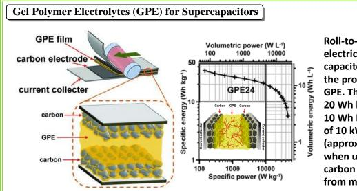
Roll-to-roll assembly of electric double-layer capacitors (EDLCs) using the proposed solid-state GPE. The GPE EDLC delivers 20 Wh kg<sup>-1</sup> (approximately 10 Wh L<sup>-1</sup>) at a high power of 10 kW kg<sup>-1</sup> (approximately 5 kW L<sup>-1</sup>) when using a high-porosity carbon electrode derived from mesophase pitch.
