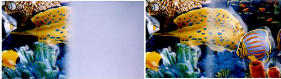
Liquid crystals can be used for LC display. Voltage bias changes LCD from "OFF" state to "ON" state. The response time could be really fast.
