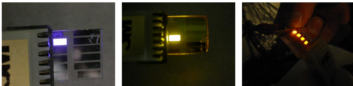
Figure 3. Photographs of PLED Devices with emitting layer are : (a) polyfluorene (b) SY-PPV on ITO glass and (c) MEH-PPV on flexible substrate, the area of each dot is 4 \text{ mm}^2
