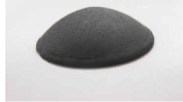
Free-standing diamond films for high-frequency diaphragms for speakers
