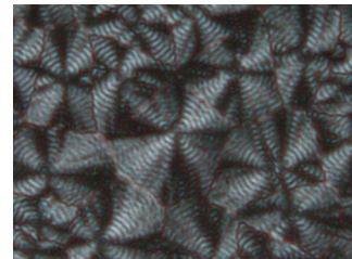
Polarized optical microscopy of PE showing spherulites with ring structure.
