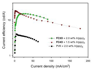
Two new bipolar compounds (FC3O, FC4O) were synthesized and applied as hosts for phosphorescent organic light-emitting diodes, using spin-coating process to cast homogeneous emission layer. Their device performances outperform conventional polymeric host PVK.
