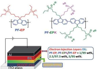
Copolyfluorenes containing pendant phosphonate groups (**PF-EP**) or partially hydrolyzed phosphonate groups (**PF-EPK**) were prepared and applied as electron-injection layer. They significantly enhance the performance of PLEDs depending on the percentage of **PF-EPK**.
