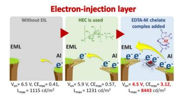
Hydroxyethyl cellulose (HEC) composited with EDTA-M (M: metal ions) chelate complexes was prepared and applied as an effective electron-injection layer in PLEDs, resulting in about 6~7 times enhancement in luminance and current efficiency.
