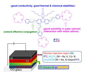
Novel azacrown-containing fluorene derivative applied (FTC) was prepared and as electron-injection layer (EIL) in polymer light-emitting diodes (PLEDs). When doped with carbonates and metal metal acetates, it significantly enhances device performance of PLEDs with PF-Green-B or Super Yellow (HY-PPV) as emitting layer.
