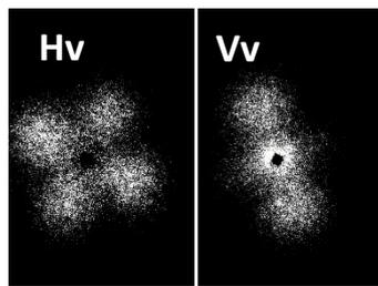
Hv and Vv patterns of sPS at 120°C by small-angle light scattering.
