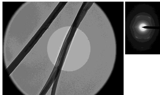
TEM image of sPS nanofibers. Inset: electron diffraction pattern
