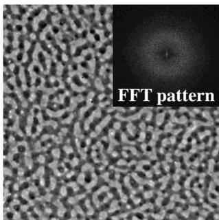
Phase separation of sPS/iPS at 300°C.
