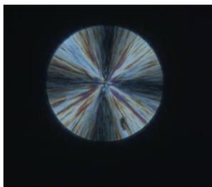
iPS spherulite observed under POM.
